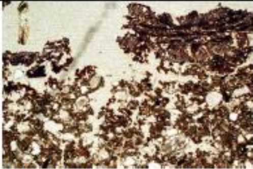
Fig. 12: As Fig 8, showing wood remains on surface of compact floor 'silts' (see Fig 2); note humification and extremely thin organic excrements along this junction testifying to wood (plank?) decay. PPL, frame width is ~4.62mm.
